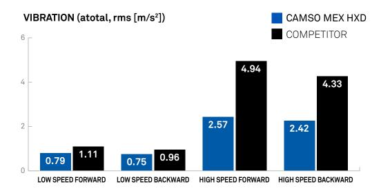
Throughout the entire test, the vibration level was 42% lower with the Camso tracks than the OEM quality track regardless the speed and the direction.
