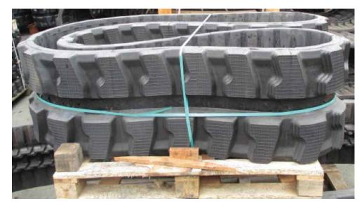
If the tracks stay palletised like this during a long time, at the moment of the fitting on the machine it will create vibration issue due to wave shape. This problem will be accentuated if the weather is cold.
