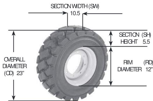
\* Industrial wheels and rims are not all the same. When calculating a tire size for polyurethane flat proofing material, drop center wheels require additional material over standard wheels.
